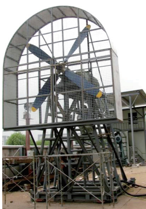
幕墙动风压装置 Air Craft Engine (最大风速50m/s) (Capable of Producing A Wind Velocity In 50m/s)— Dynamic Water Permeability Test
