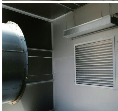
通风防雨百叶、防沙百叶测试装置 Testing Equipment for Wind Driven Rain Performance and Subjected to Sand Performance of Louvres
